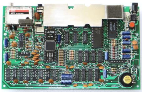
Fig.2 - vLA82 installed
