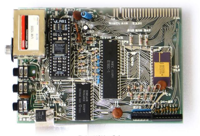
Fig.1 - vLA81 installed
