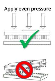
Do NOT bend PCB or insert at an angle
