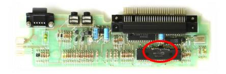
The next task is to remove the existing ULA without damaging the PCB. The tracks are very narrow and excess heat or trying to remove the IC before the pins are free of solder will guarantee that the tracks will lift. If the existing ULA is known to be faulty then the IC pins can be snipped close to the IC body and each pin removed separately. If the existing ULA is still OK then proceed with caution and make sure all pins are free before attempting removal!
